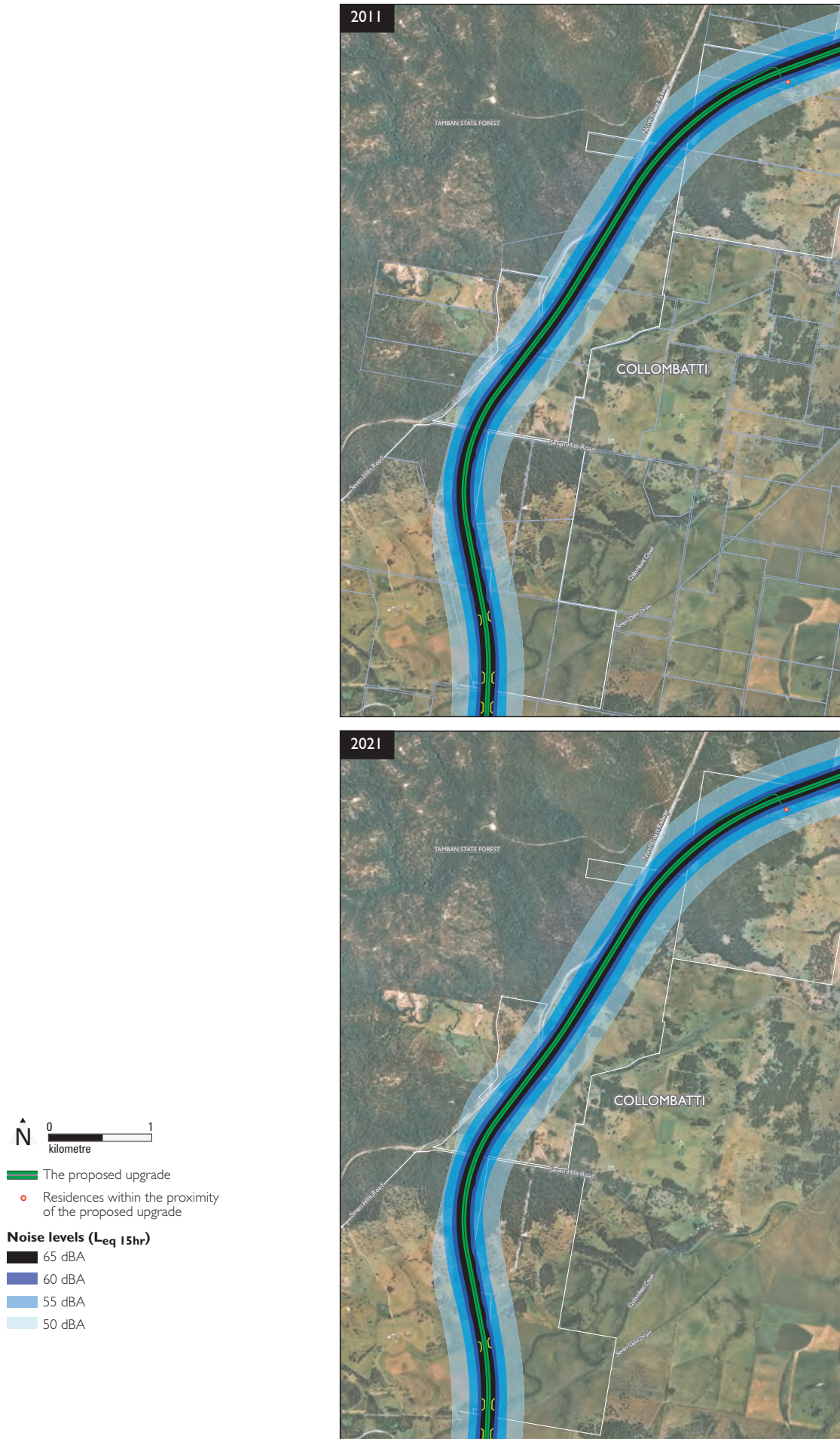
Figure 16-8 2011 and 2021 daytime noise impacts – Collombatti North
