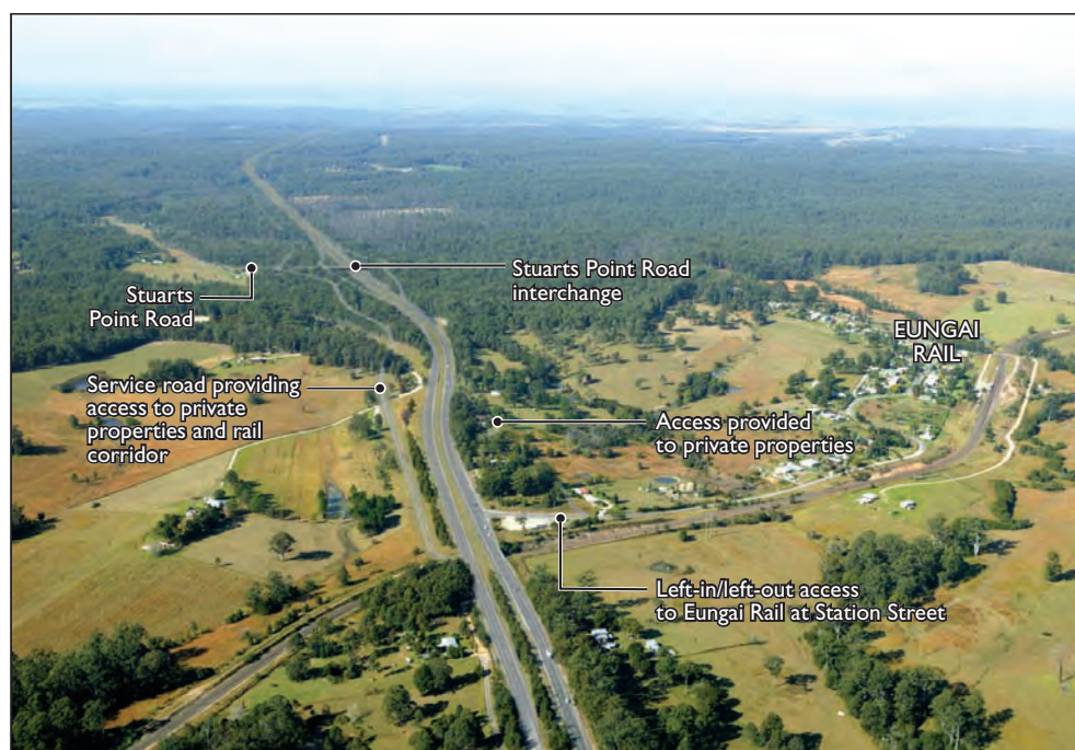
Figure 6-6 Photo-illustration of the proposed Stuarts Point Road interchange (looking south)
