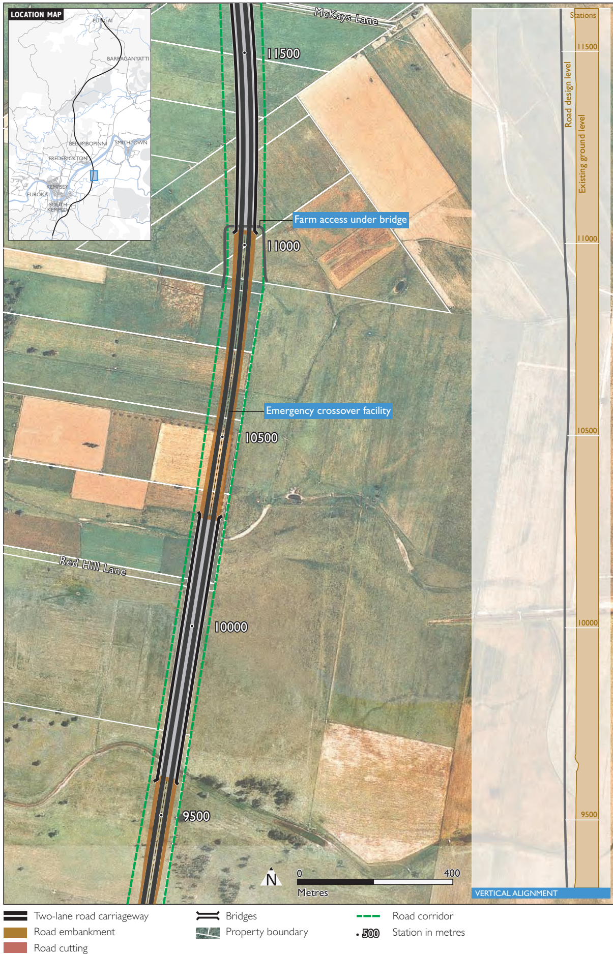
Figure 6-1f Horizontal and vertical route alignment
