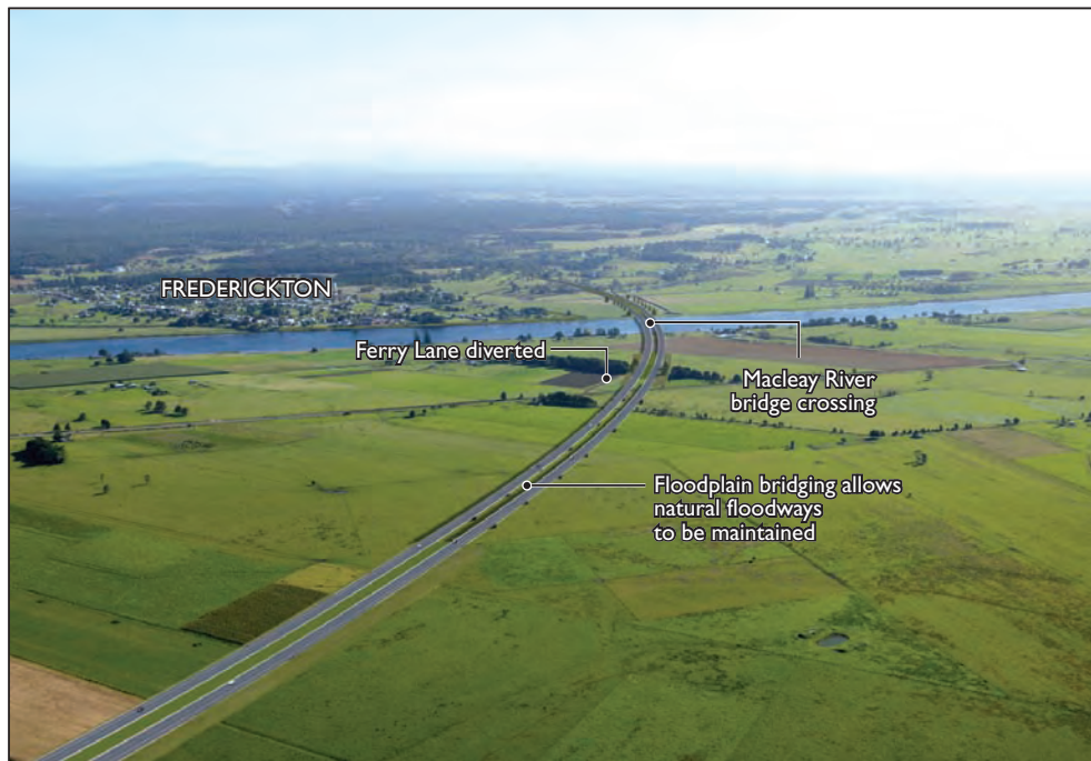
Figure 6-8 Photo-illustration of the proposed floodplain bridging at Frogmore (looking west)
