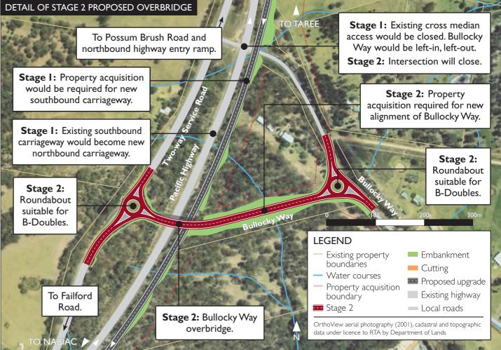
The existing highway intersections at Possum Brush Road and Tritton Road would close in Stage 1, and Bullocky Way would become left-in, left-out. Bullocky Way intersection would close in Stage 2.
