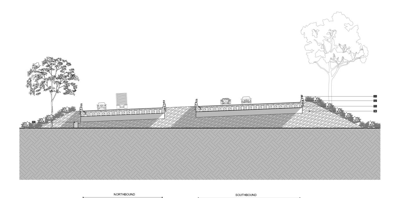
Figure D.3.15.2 Twin Bridges over Water Course and Fauna Crossing: Cross Sectional Elevation
