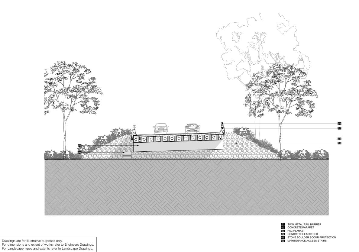
Figure D.4.3.2 Service Road Bridge over Water Course and Fauna Crossing: Cross Sectional Elevation
