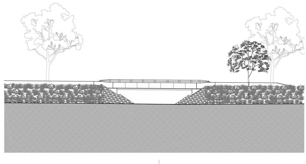
Figure D.3.15.1 Twin Bridges over Flow Balancing Water Course and Fauna Crossing: Elevation
