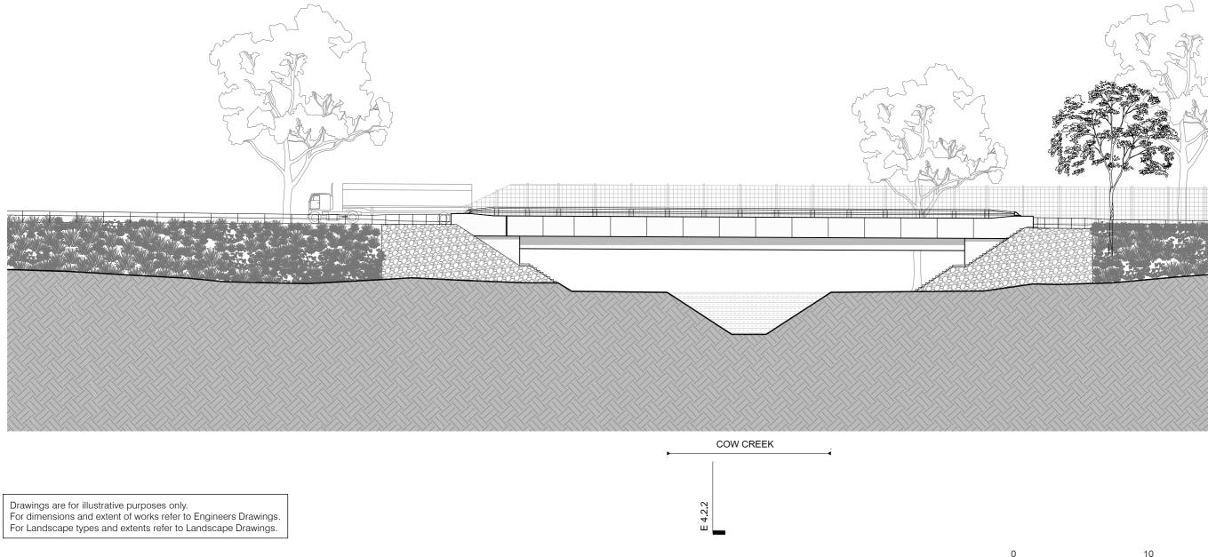
Figure D.4.2.1 Service Road Bridge over Cow Creek - Elevation
