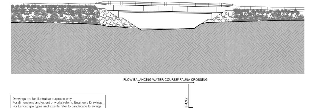
Figure D.4.3.1 Service Road Bridge over Water Course and Fauna Crossing - Elevation
