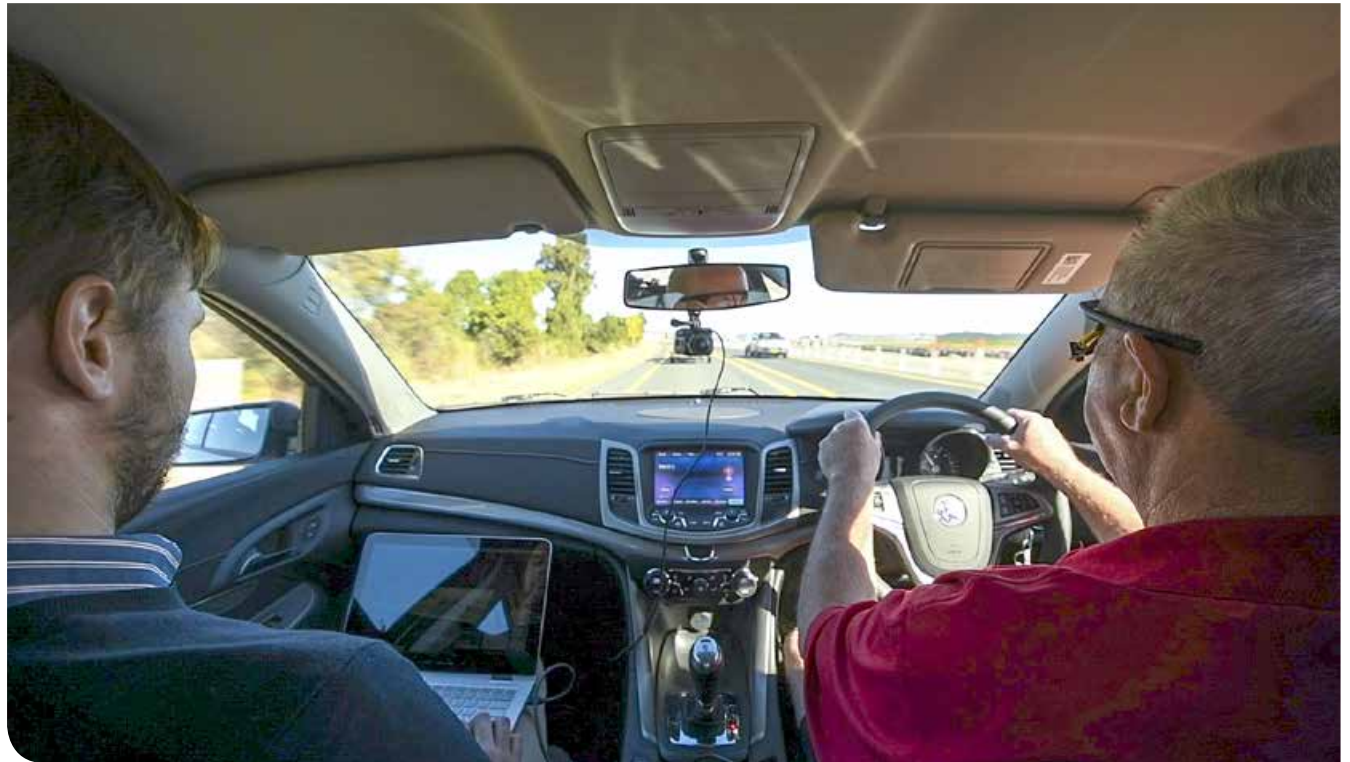
A participant being monitored with video, audio, GPS and eye-tracking devices as part of the Driver Safety Study conducted on the Pacific Highway between Iluka and Maclean
