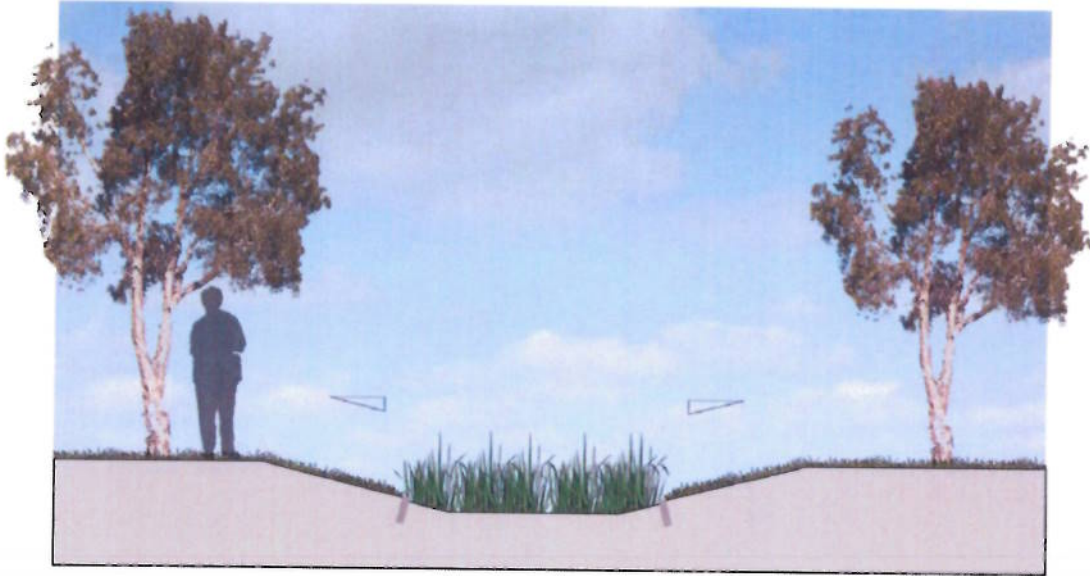
Figure 1. An example of the use of swales for flow conveyance and water quality improvement.
