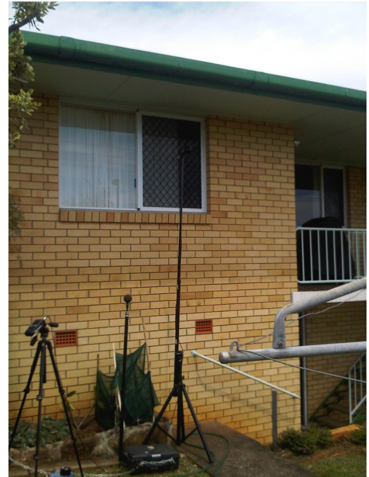
Concurrent short term (attended) noise measurements
