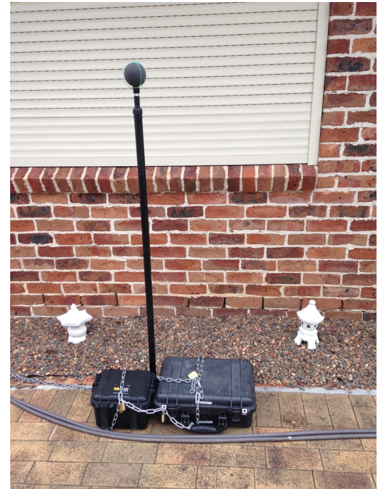
Long term (unattended) noise monitor at 1m from facade
