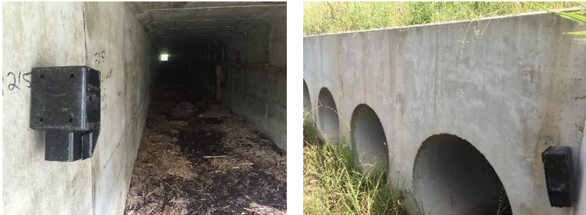
Plate 12: Single cell underpasses were monitored at each end with a Reconyx HC500 camera housed in a security case and mounted to the side wall opposite the wooden rail (e.g. Moonee underpass, Left). For the pipe series at Emerald Beach, a camera was mounted on the wing wall at either side of the pipe series and directed across the entrance area on the east side (Right).
