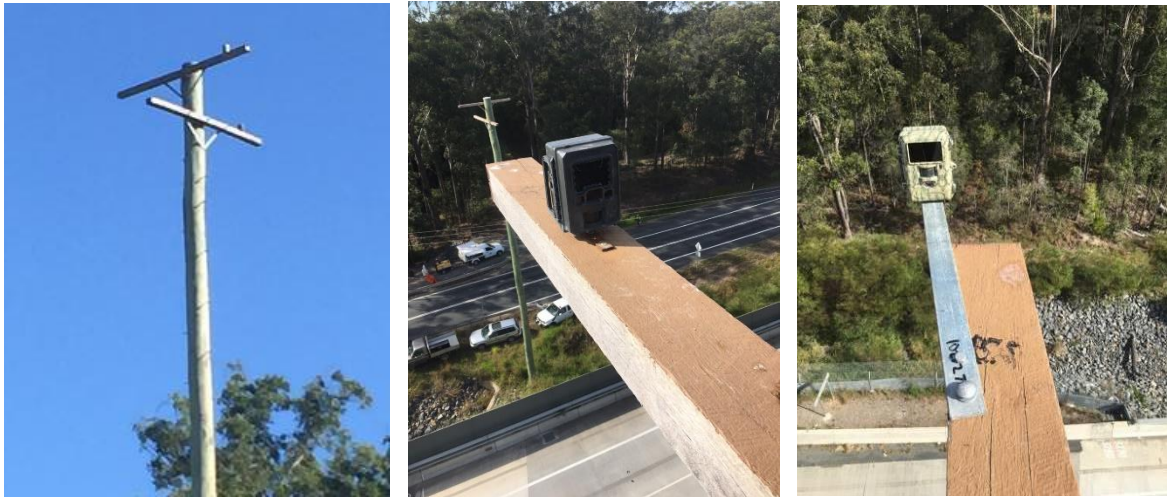
Plate 17: Year 1 and early Year 2 glide pole monitoring featured an SC950 Reconyx camera mounted to the east end of the upper arm and the north end of the lower arm (Left & Middle). During year 2 monitoring (18/5/2016) a Scoutguard KG680V was installed on the end of a flat bar at the opposite end of each arm to the Reconyx cameras (Right).
