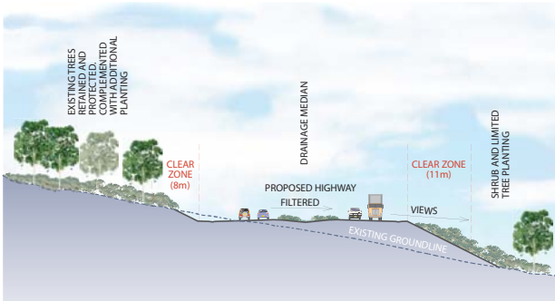
Illustration 76: Cross section at chainage 143,700
