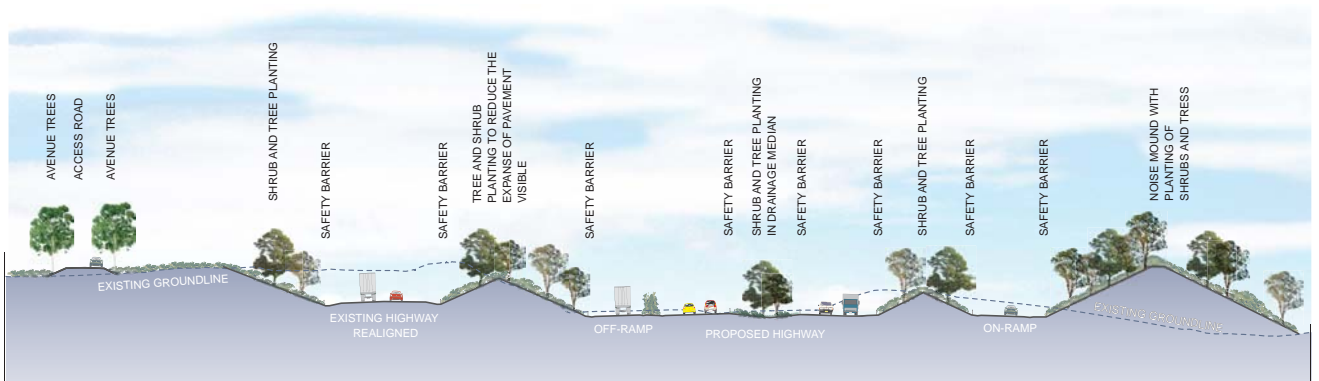
Illustration 87: Cross section at chainage 151,800
