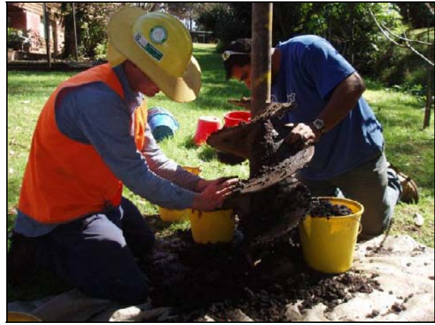
Transferring deposit from auger blade to buckets
