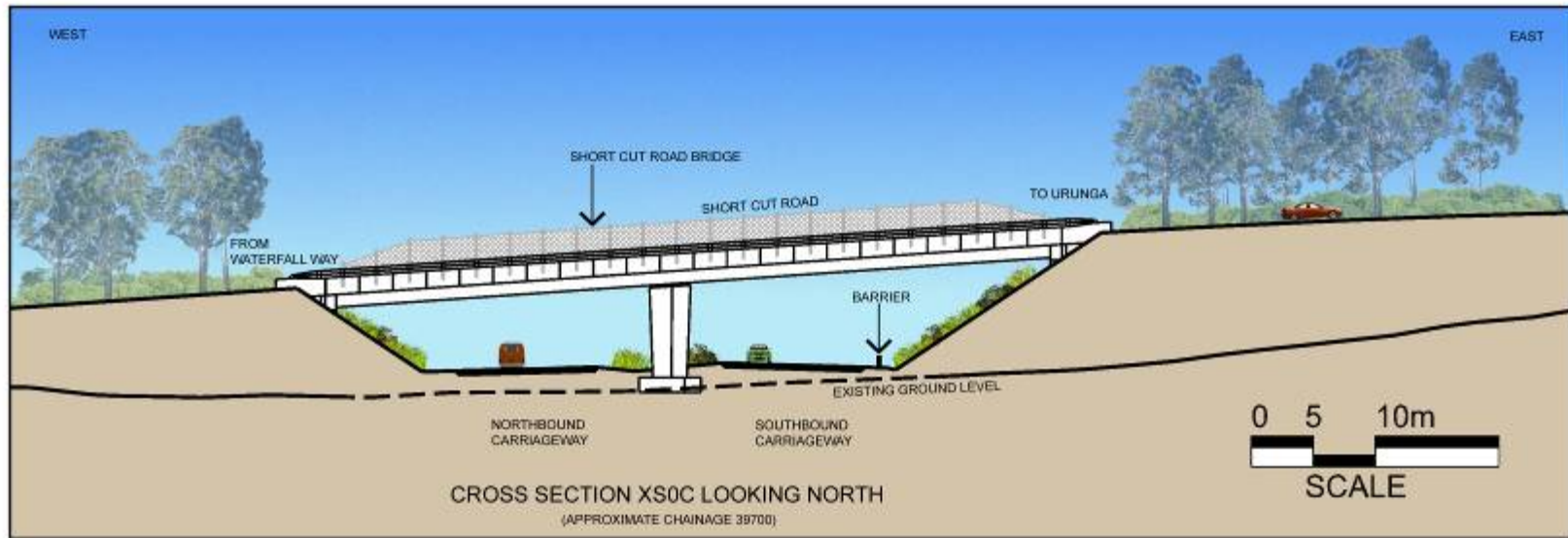
Figure 6-19 C/S XS0C Typical cross section at Short Cut Road looking north (approximate chainage 39700 m)
