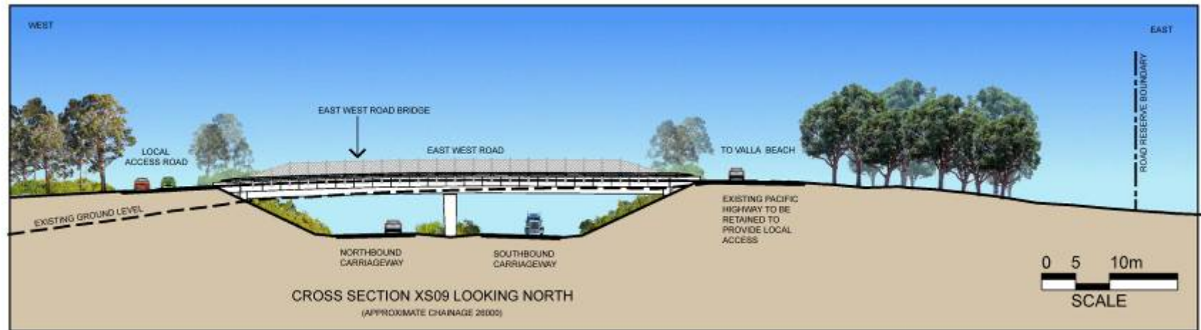
Figure 6-17 C/S XS09 Typical cross section at East West Road looking north (approximate chainage 26000 m)
