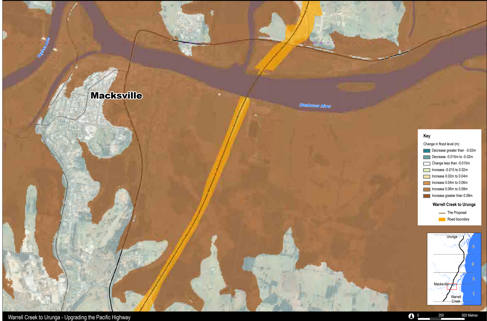
FIGURE 16-8b | NAMBUCCA RIVER - DEVELOPED CONDITIONS WITH CLIMATE CHANGE IMPACTS 100 YEAR ARI FLOODING (OPTION 2)
