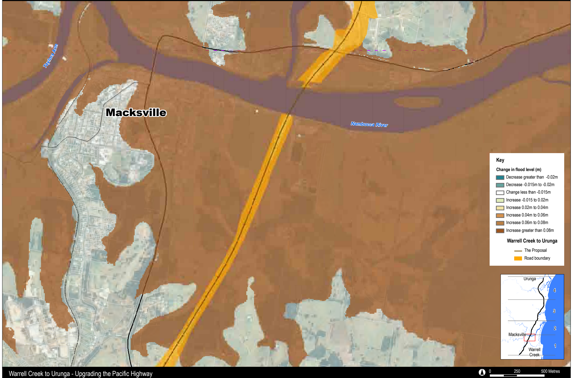
FIGURE 16-8a | NAMBUCCA RIVER - DEVELOPED CONDITIONS WITH CLIMATE CHANGE IMPACTS 100 YEAR ARI FLOODING (OPTION 1)
