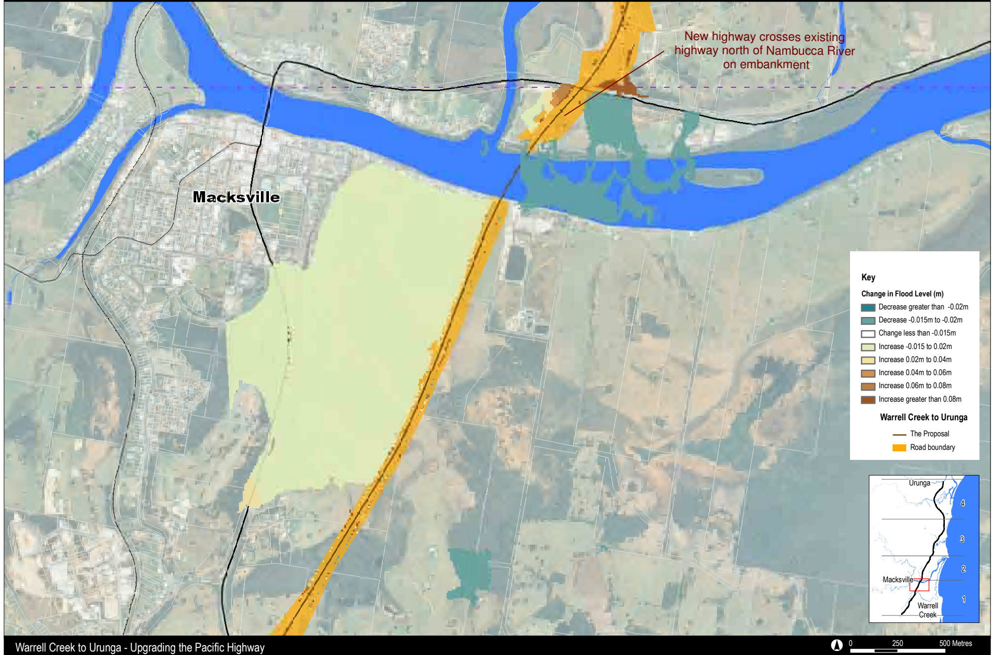
FIGURE 16-4a | NAMBUCCA RIVER - DEVELOPED CONDITIONS 100 YEAR ARI CHANGE IN FLOOD LEVEL (EMBANKMENT OPTION)
