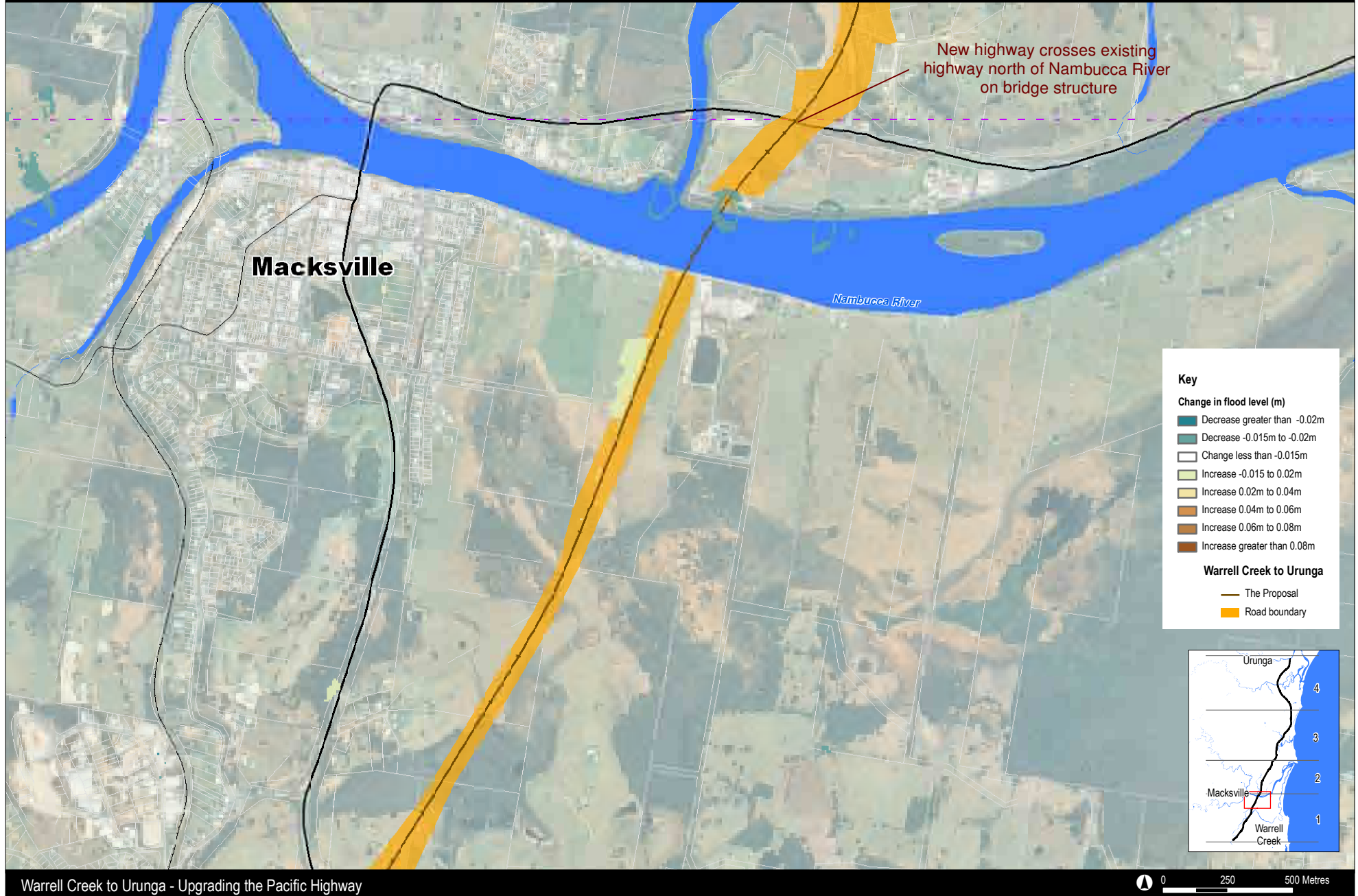
FIGURE 16-4b | NAMBUCCA RIVER - DEVELOPED CONDITIONS 100 YEAR ARI CHANGE IN FLOOD LEVEL (BRIDGE OPTION)
