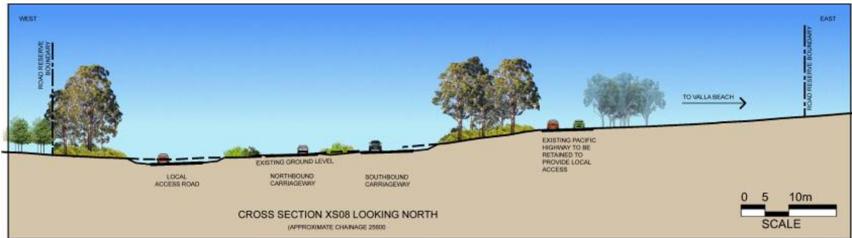
Figure 6-16 C/S XS08 Typical cross section near Valla Beach looking north (approximate chainage 25600 m)
