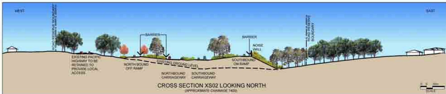
Typical Cross Section at Bald Hill Road Interchange looking North (Approximate Chainage 7400)
