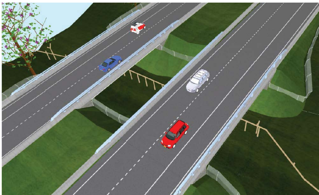
Fig 3. 3D Model of typical 15m plank bridges for koala connectivity- note twin bridges and daylighting in the median
