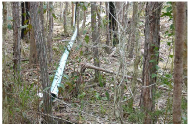
Pipe from sediment basin diverts water into quadrat June 2016
