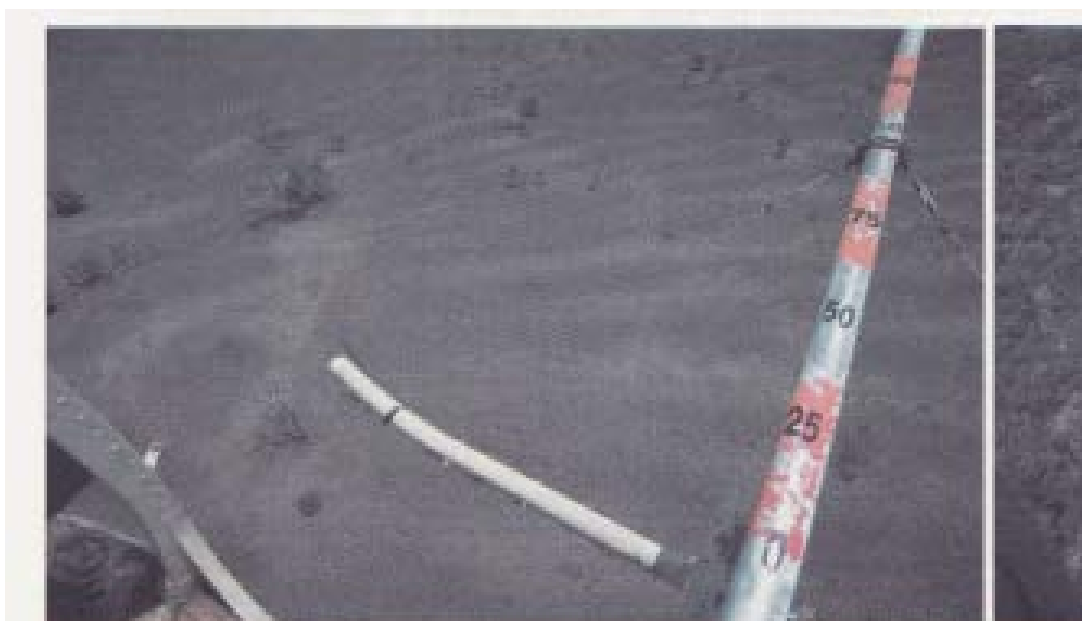
Figure 1. Example of pole used to delineate distances of observations from the transect
