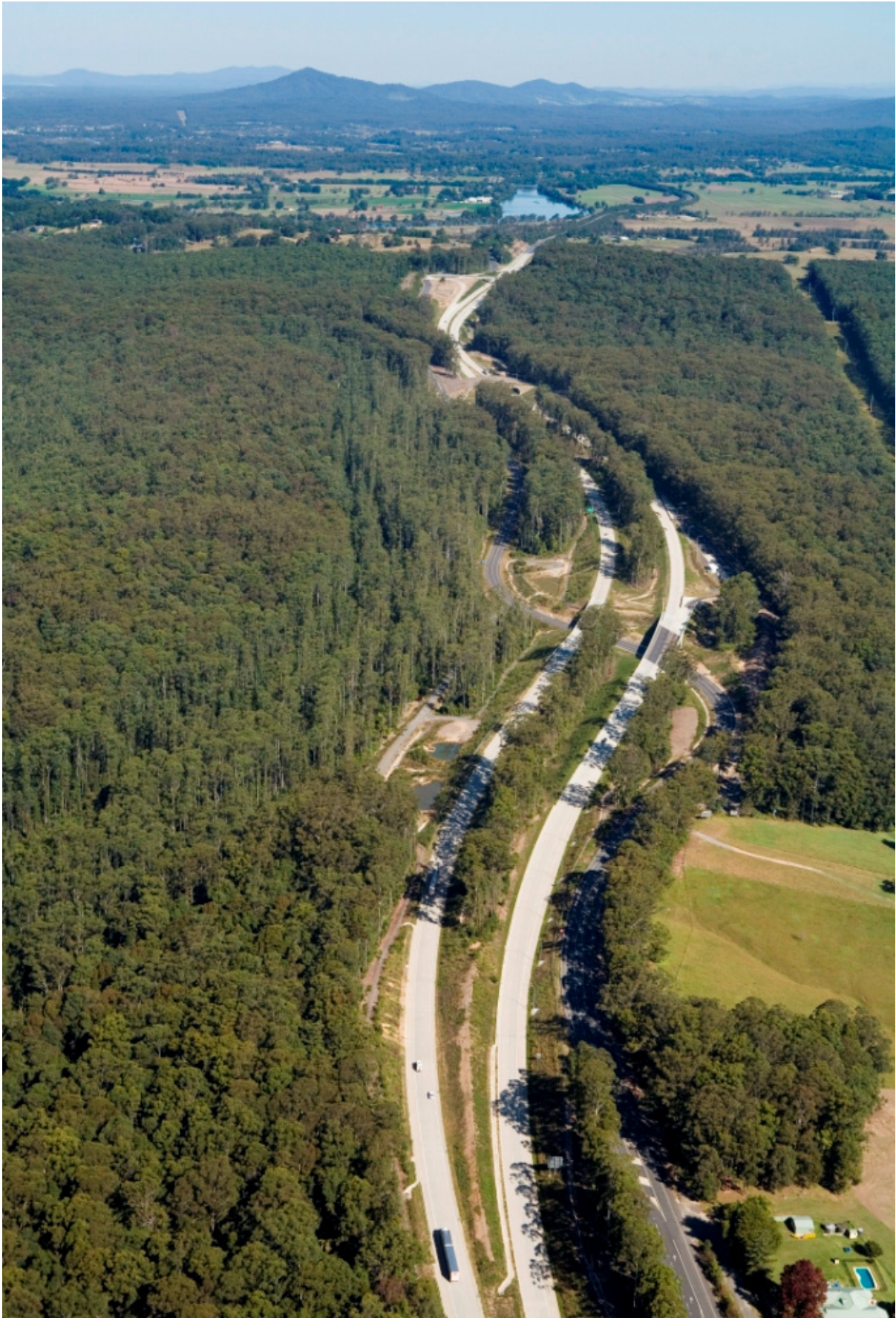
Photo 3: Pacific Highway at Bonville upgrade showing median widening for fauna connectivity
