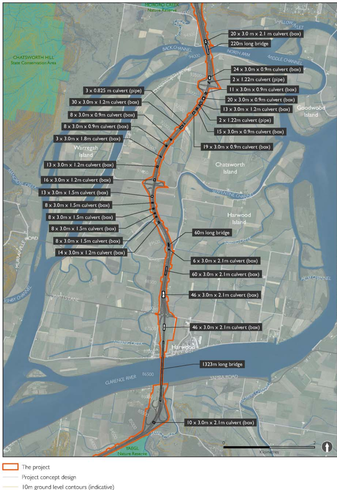
Figure 5-108: Location of typical flood relief structures- Chatsworth Island floodplain
