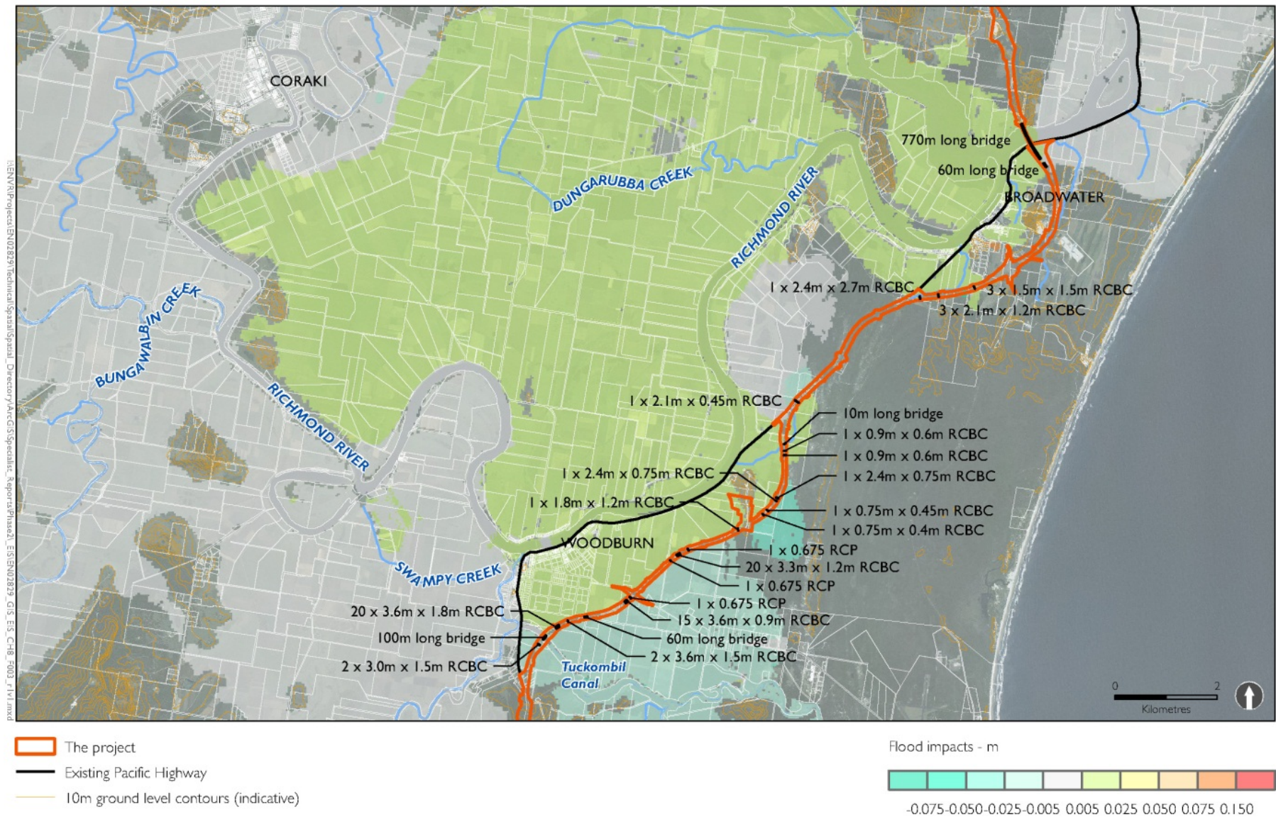
Figure 8-8: Flood impacts 20 year ARI flood event: mid Richmond River
