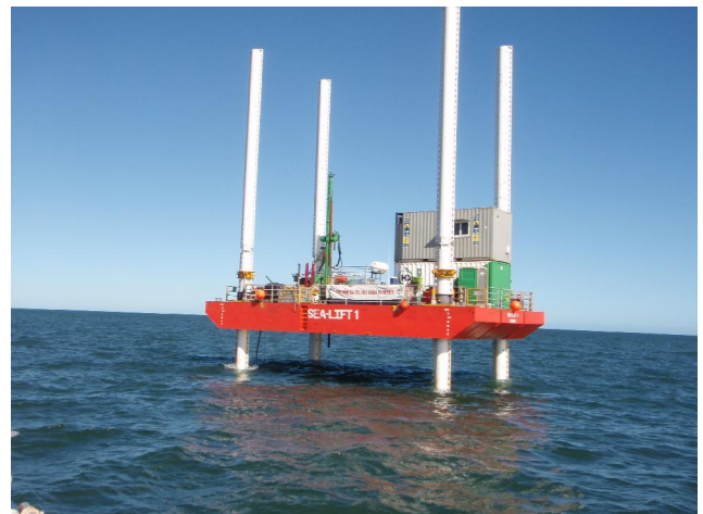
A barge and geotechnical drill equipment
