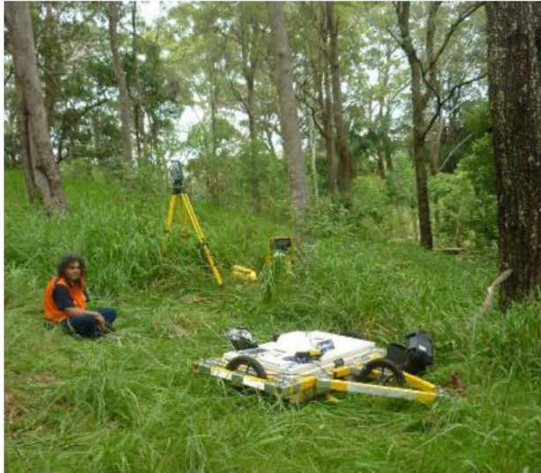
Image 2: MALA MIRA system and Trimble Total Station
