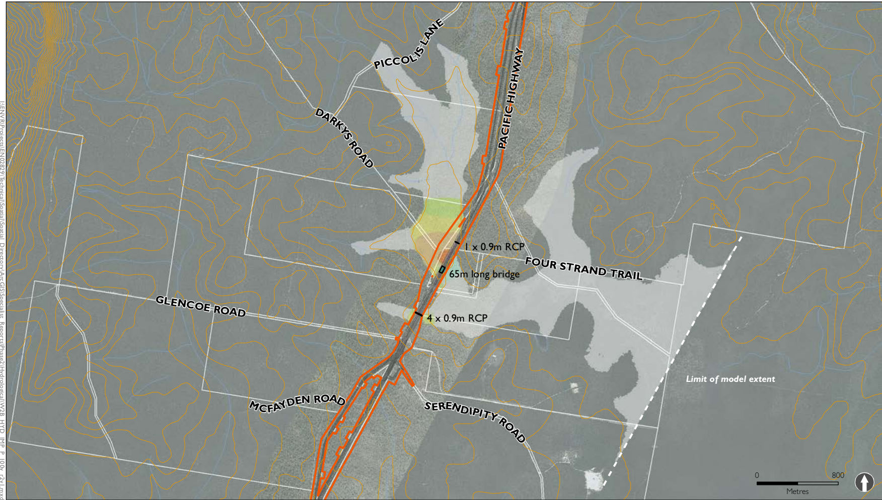
Figure 6-36 Flood impacts 100 year ARI event: Tabbimoble Floodway No. 1
