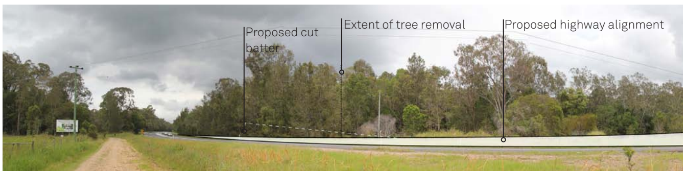
Annotated diagrammatic approximation of the project as photographed from viewpoint 39_ View south-east Pacific Highway, south of Woodburn. Location: 29°05'48"S 153°20'23"E
