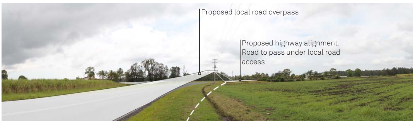
Annotated diagrammatic approximation of the project as photographed from viewpoint 42_ View south-east Evan Head Road, Woodburn. Location: 29°04'40"S 153°04'64"E
