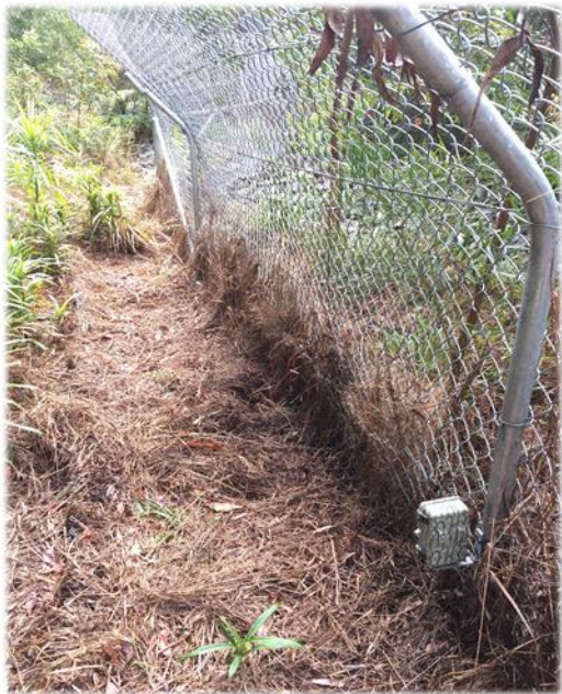
Plate 3: Typical exclusion fence camera installation. A Scoutgaurd KG680V mounted on a steel bracket attached to fence post.
