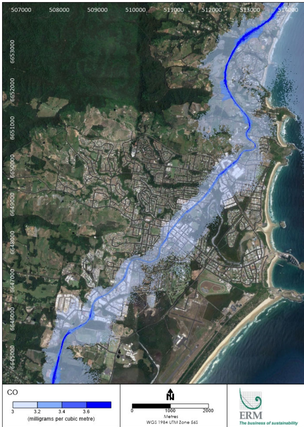
Figure C-8: Predicted maximum 8-hour rolling average cumulative CO concentrations for 2024 – No Build ( \mu\text{g}/\text{m}^3 )
