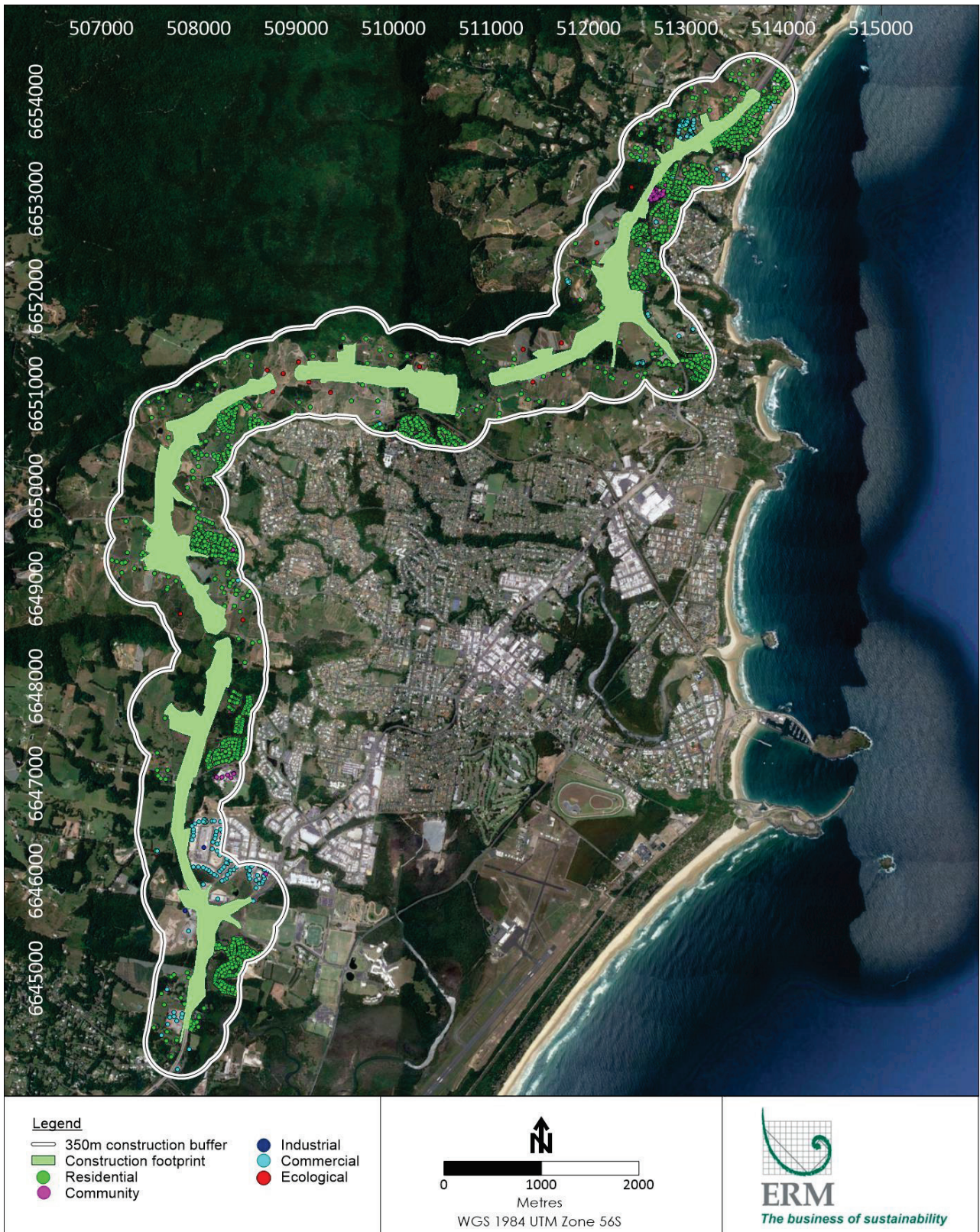
Figure 4.1: Receptors evaluated for construction air quality impacts (ERM 2019)
