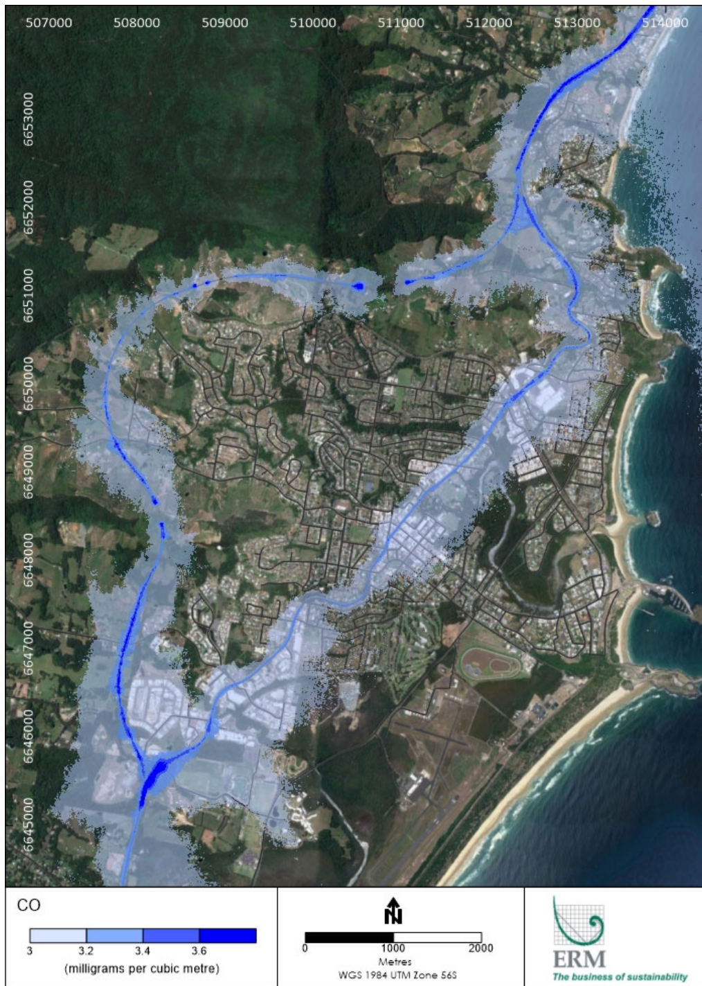
Figure C-16: Predicted maximum 8-hour rolling average cumulative CO concentrations for 2024 – Build ( \mu\text{g}/\text{m}^3 )
