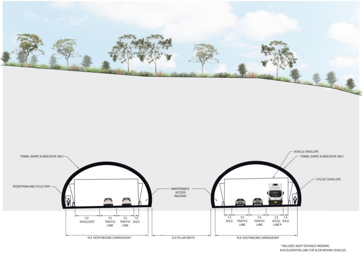
Figure 5-6 Tunnel typical cross section
