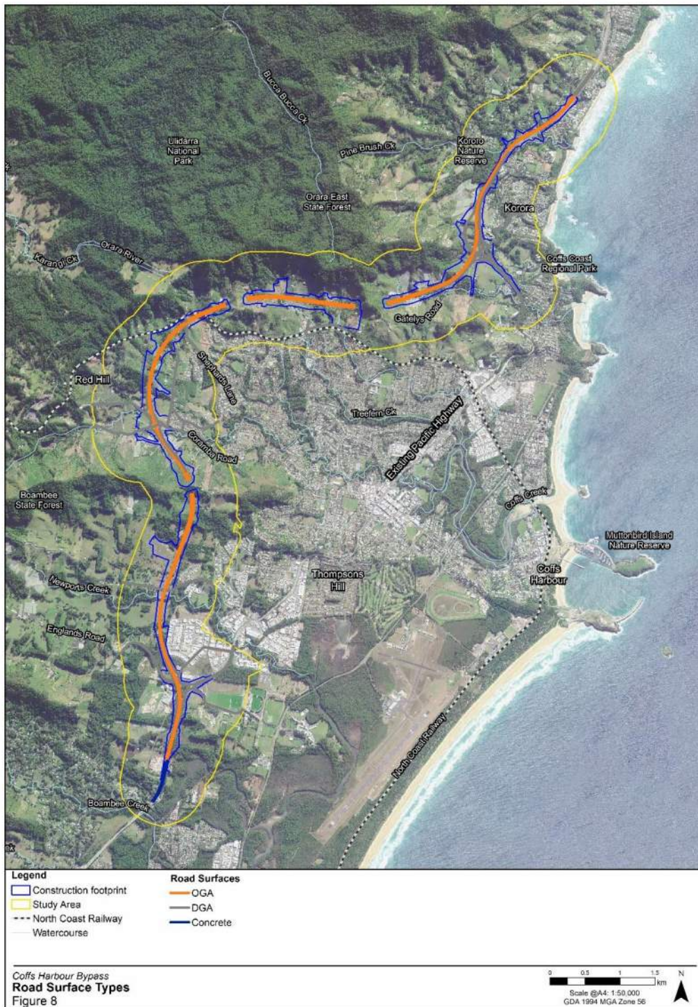
Figure 8: Extents of low noise pavement along the bypass
