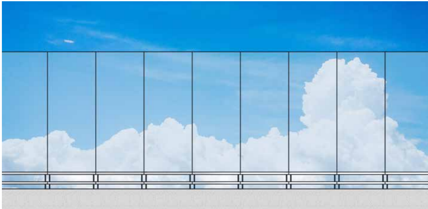
FIG 5.17 TYPICAL ELEVATION TRANSPARENT NOISE WALLS
