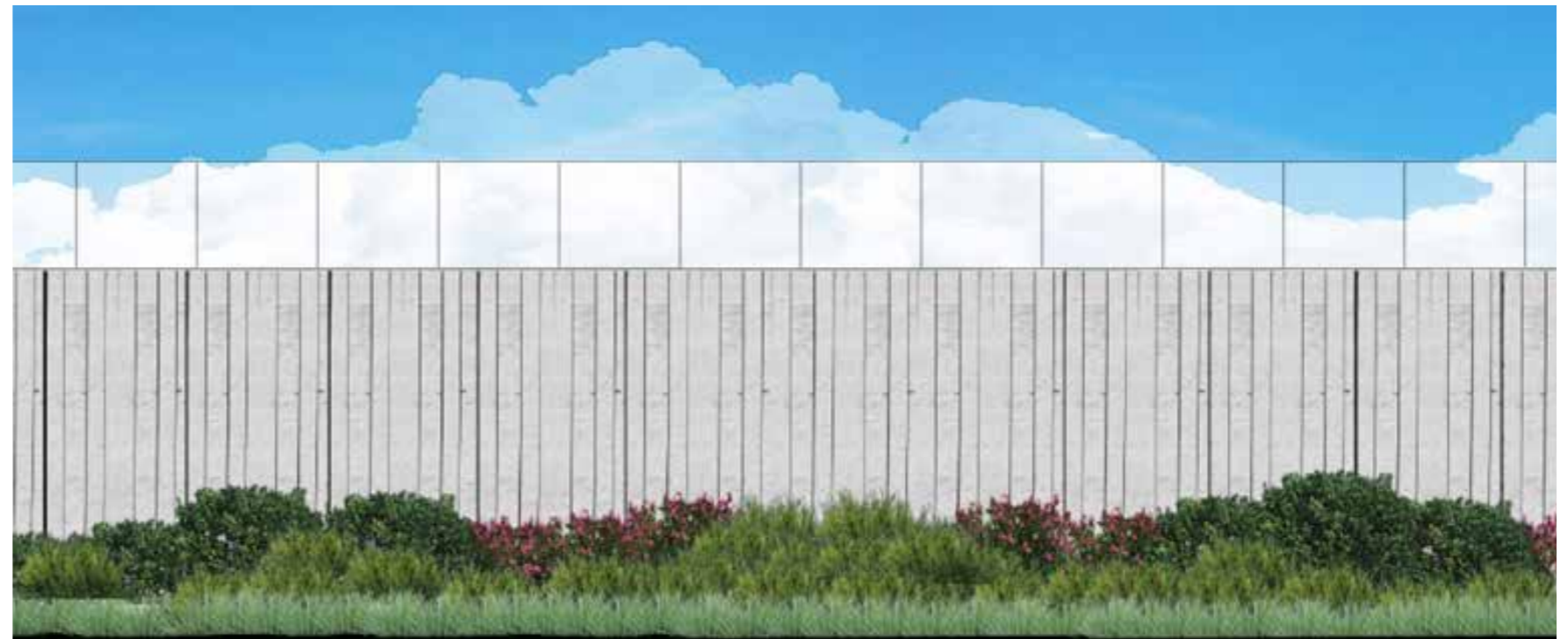
FIG 5.15 TYPICAL ELEVATION TRANSPARENT CLEAR PANEL ABOVE SOLID WALL
