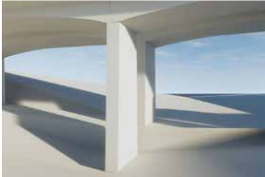
FIG 5.31 PIER OPTION 5 - TAPER
