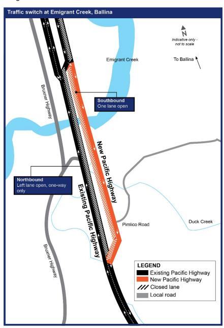
These traffic changes will allow us to maintain traffic flow on the road network while we safely continue to build the upgrade and will remain in place as drainage and finishing work are carried out. Motorists will be kept informed about dates for the traffic changes through electronic message signs and on livetraffic.com.au.
