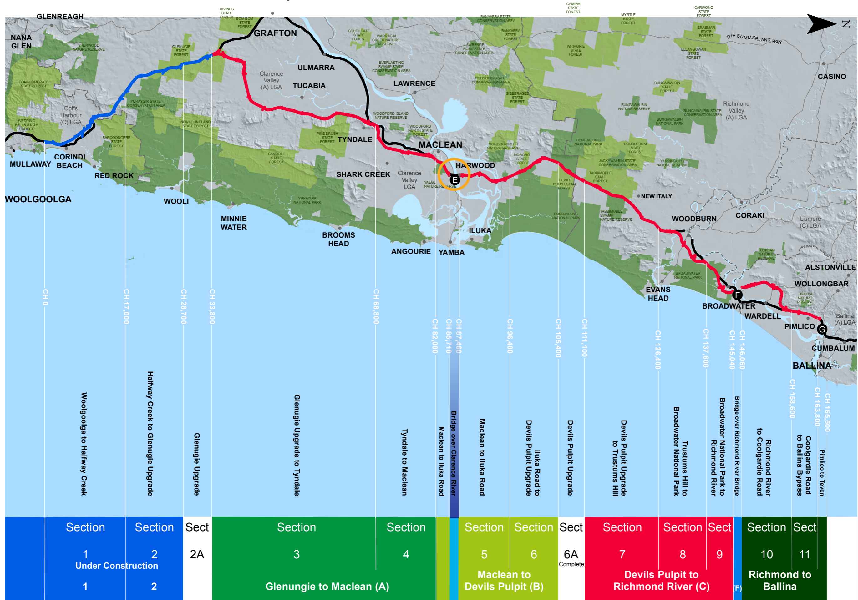
Figure 1-2: Pacific Highway Woolgoolga to Ballina upgrade Section map (source: Pacific Complete)
