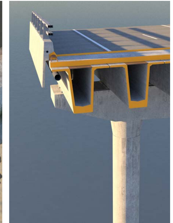
Figure 8.15 Artist impression of bridge drainage Subject to further design
