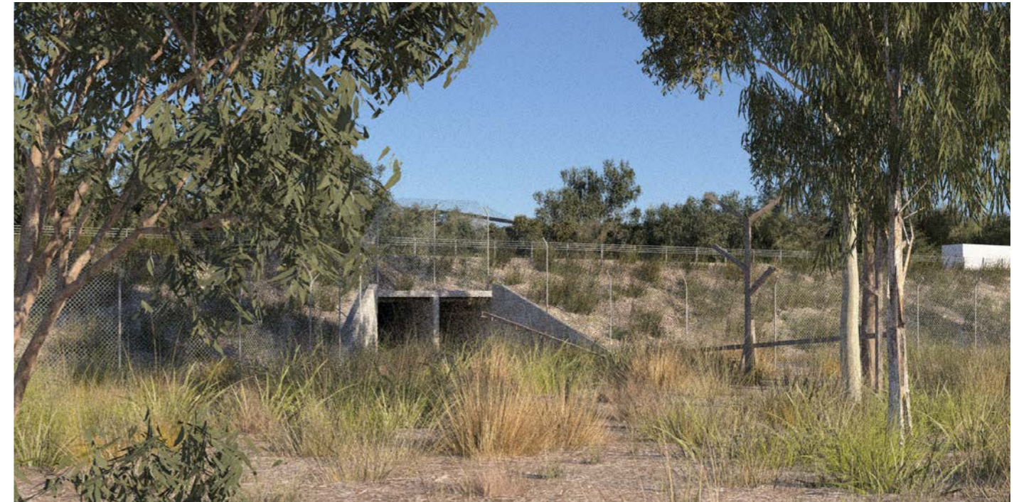
Figure 7.8 Artist impression of fauna culvert with fauna furniture, landscape shown at full maturity
