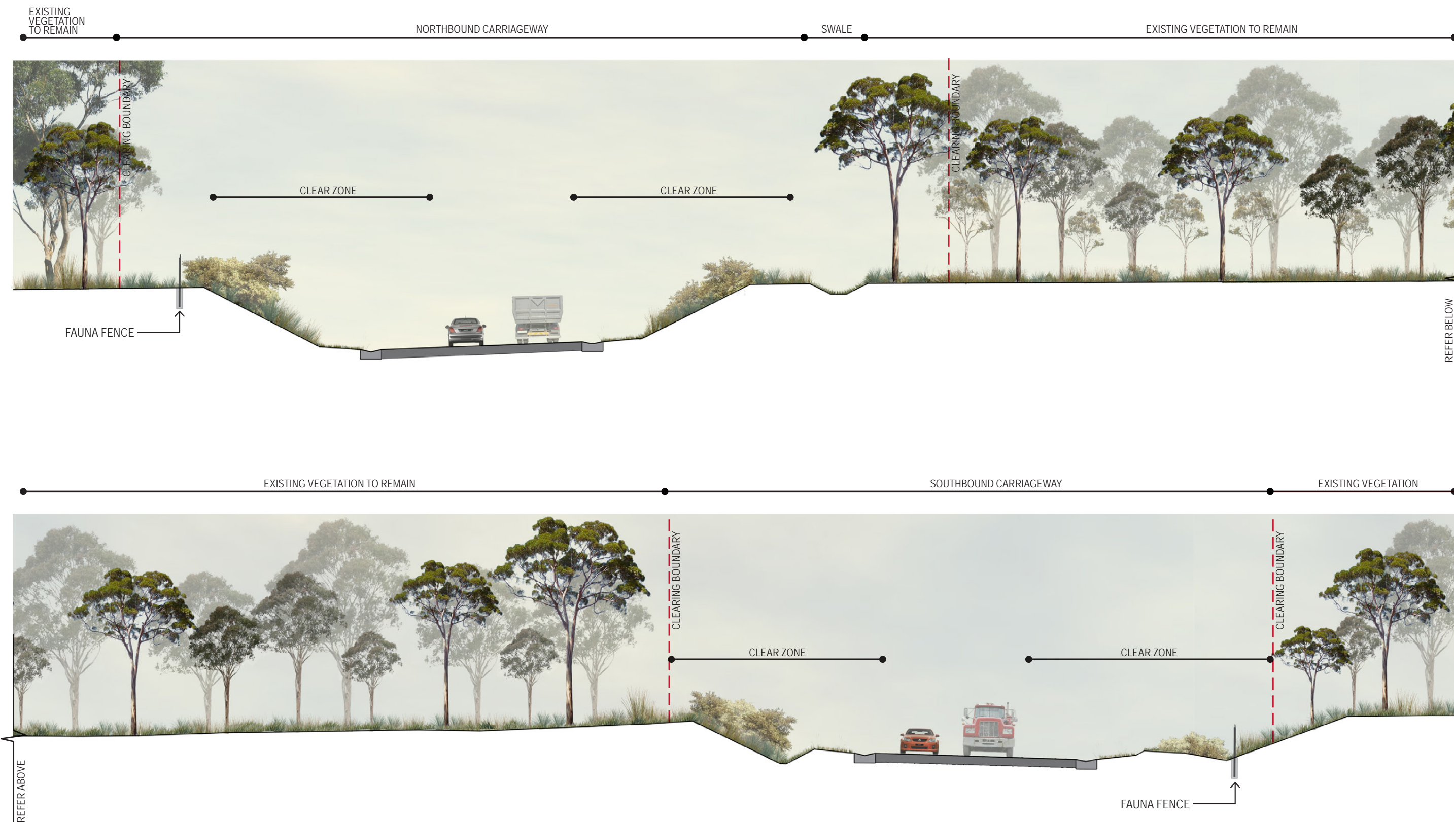
CROSS SECTION A-A CHAINAGE 117600
