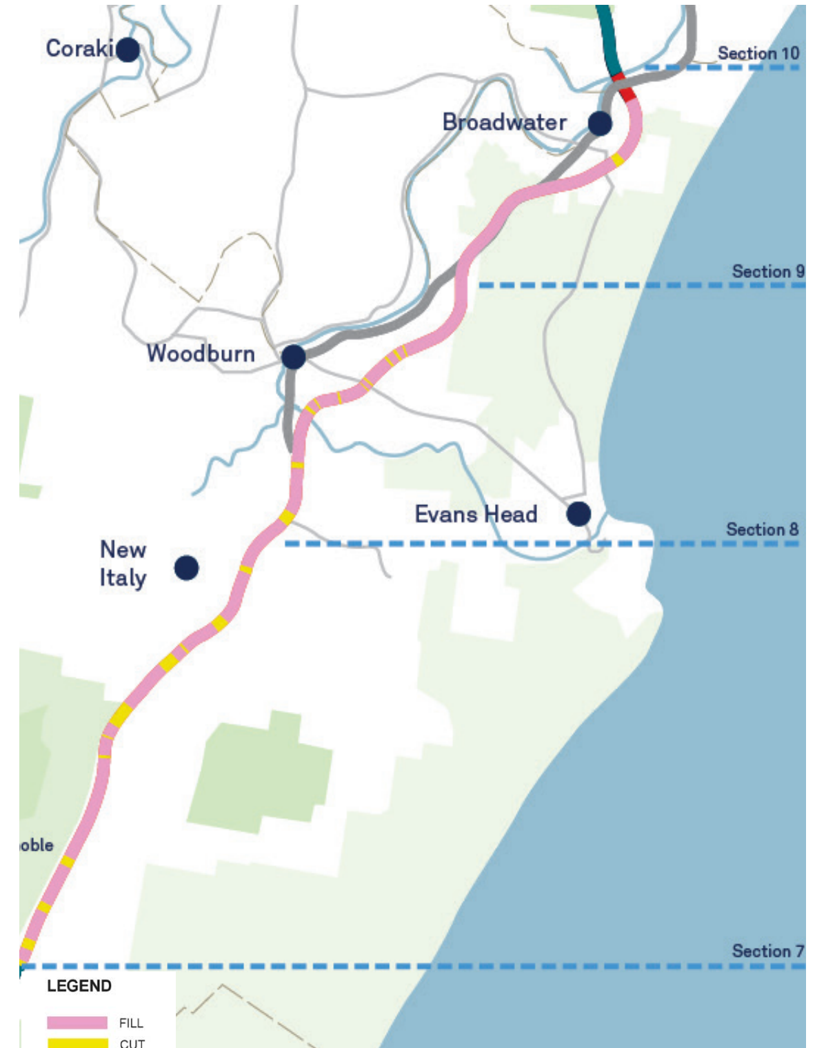
Figure 8.26 Cut and fill location map
