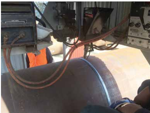
Roller and fixed welding unit in operation to weld pile casings
