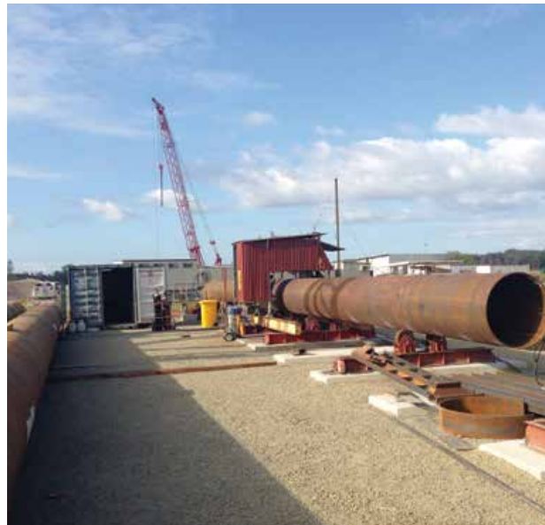
View of pile casing in place for welding with the new roller and fixed welding unit
