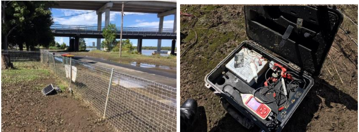
Figure 10 Noise monitoring equipment impacted by flooding event
