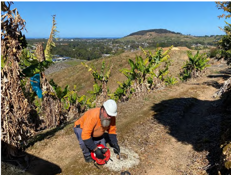
Photograph 3 , shows the use of an electronic dip meter to measure the depth to standing water at location BHH131, view is towards the east.
