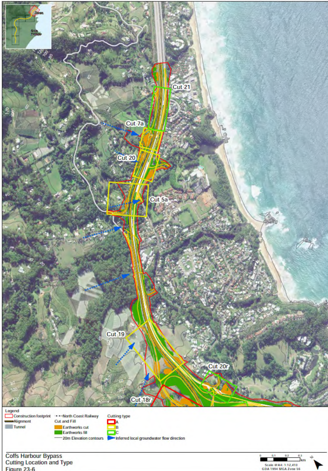
Figure 2-6: Cutting location and type - Coffs Harbour Bypass Source. TfNSW (2019), Coffs Harbour Bypass Environmental Impact Statement
