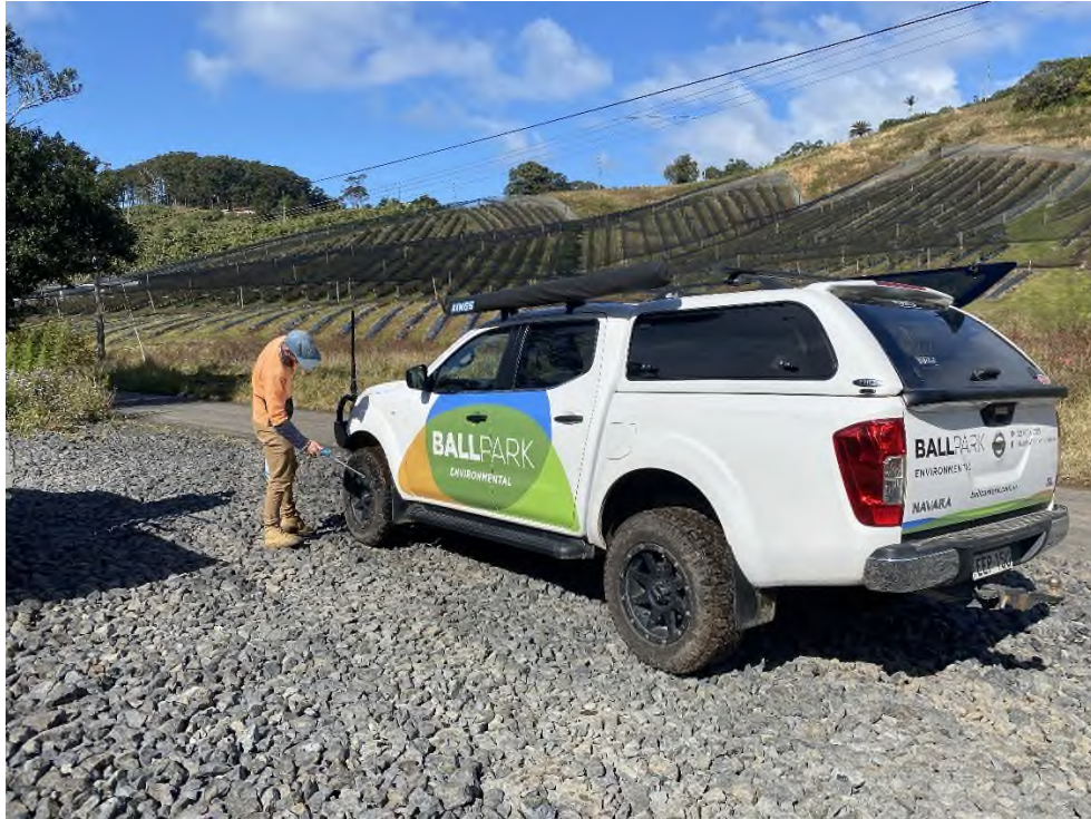
Photograph 5 , shows example of Panama disease decontamination undertaken of field vehicle using a Path X disinfectant spray. Location is the gravel wash down pad constructed to the north of Gatelys Road tunnel.
