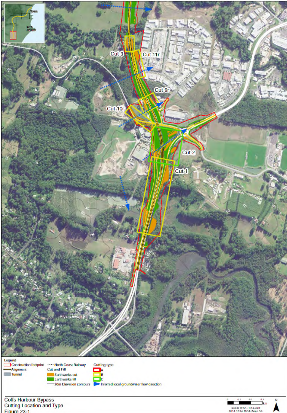
Figure 2-1: Cutting location and type - Coffs Harbour Bypass Source. TfNSW (2019), Coffs Harbour Bypass Environmental Impact Statement
