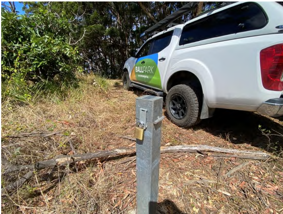
Photograph 2 , shows example of a locked monument cover at location BHH150, on the ridgeline to the west of the Gatelys Road tunnel.
