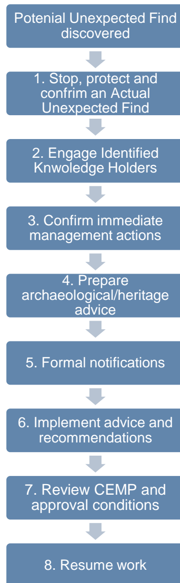
FIGURE 1 OVERVIEW OF PROCESS FOR MANAGEMENT OF UNEXPECTED FINDS
