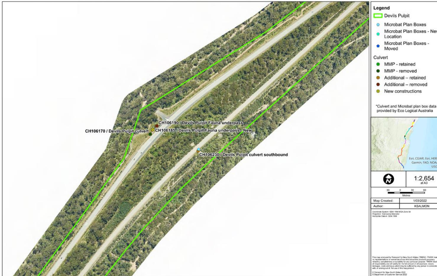
Figure 9: Devil’s Pulpit section Microbat Monitoring Plan, subject drainage structures and bat box locations.
