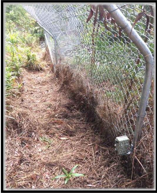
Plate 3: Typical exclusion fence camera set up. It shows a Scoutguard KG680V camera attached to a steel bracket fixed to a fence post.
